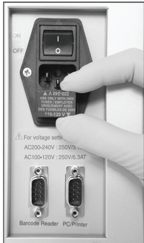
Selecting the correct fuse for 100–120 V line power supply.
